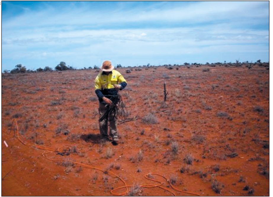
Plate 5.4 Laying of geophones during a typical 2D survey
